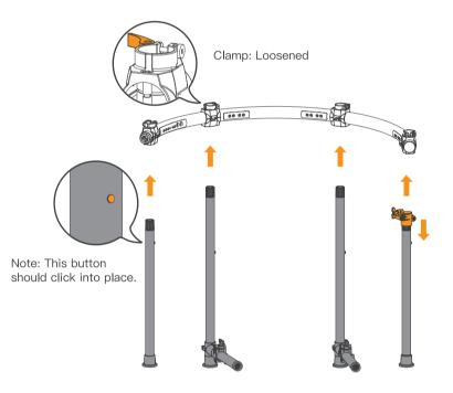
Put the drum clamps onto the two long pipes, and tighten the wing nuts.
