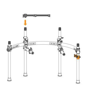
Loosen the turncap. Insert the cymbal arm into this cap as shown below, and then tighten the turncap.
