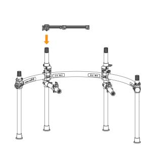
Loosen the turncap. Insert the cymbal arm into this cap as shown below, and then tighten the turncap.
