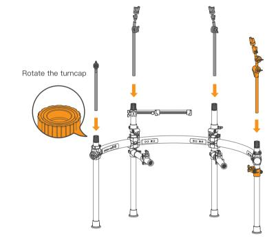
Install the L shaped HI-HAT rod and drum pad rod as shown below.
