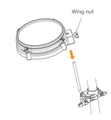
Loosen the wing nut and put the drum pad onto the L shaped pad rod. Then tighten the wing nut.
